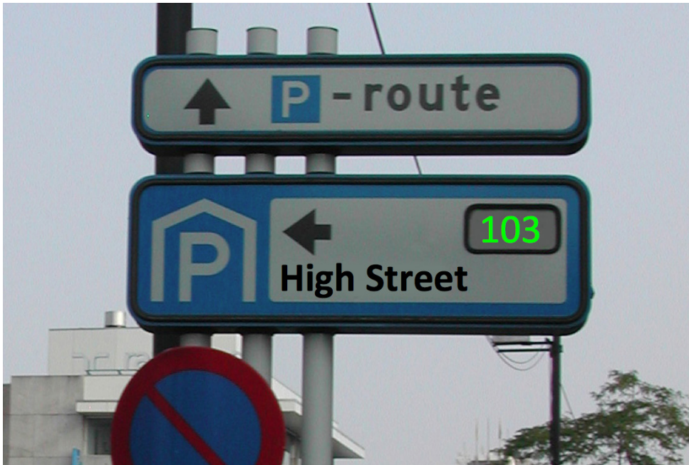
Example of a managed parking routes sign with real time information
